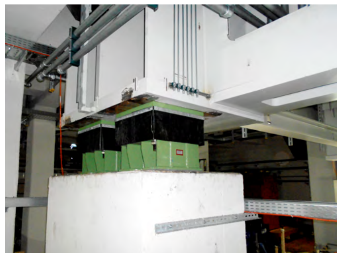
Spring Isolators for the vibration isolation of an AUDI AG press line © KTI Schwingungstechnik GmbH
