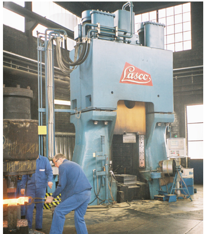
Perfectly insulated, hydraulic forging hammer
