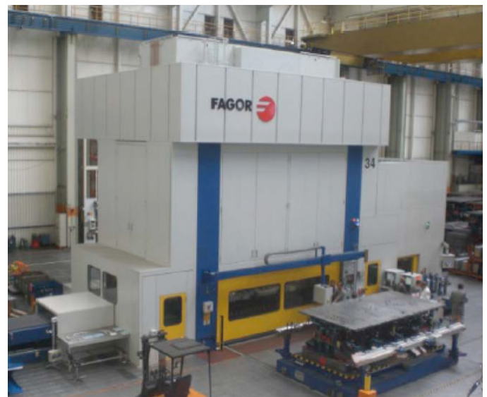
FAGOR Transfer press with a pressing force of 20,000 kN
