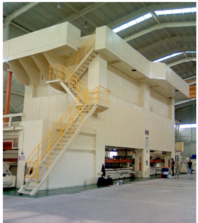
Mechanical Danly transfer press with 1,360 t gross weight
