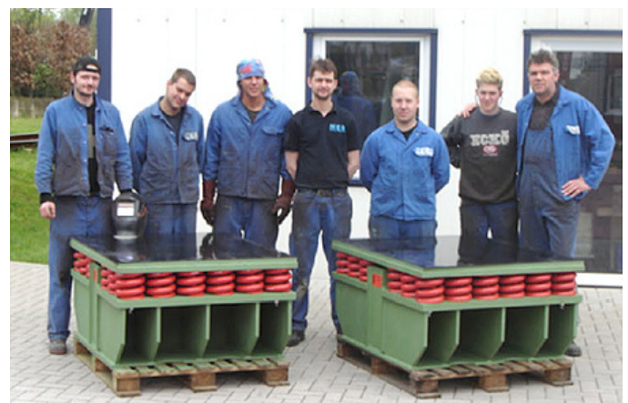
Specialists beside KTI spring supports with a load capacity of 400 t
